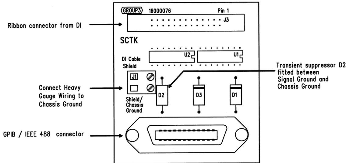
An SCR clamping structure is connected to each GPIB signal line which limits voltages on the line to below 6V.
