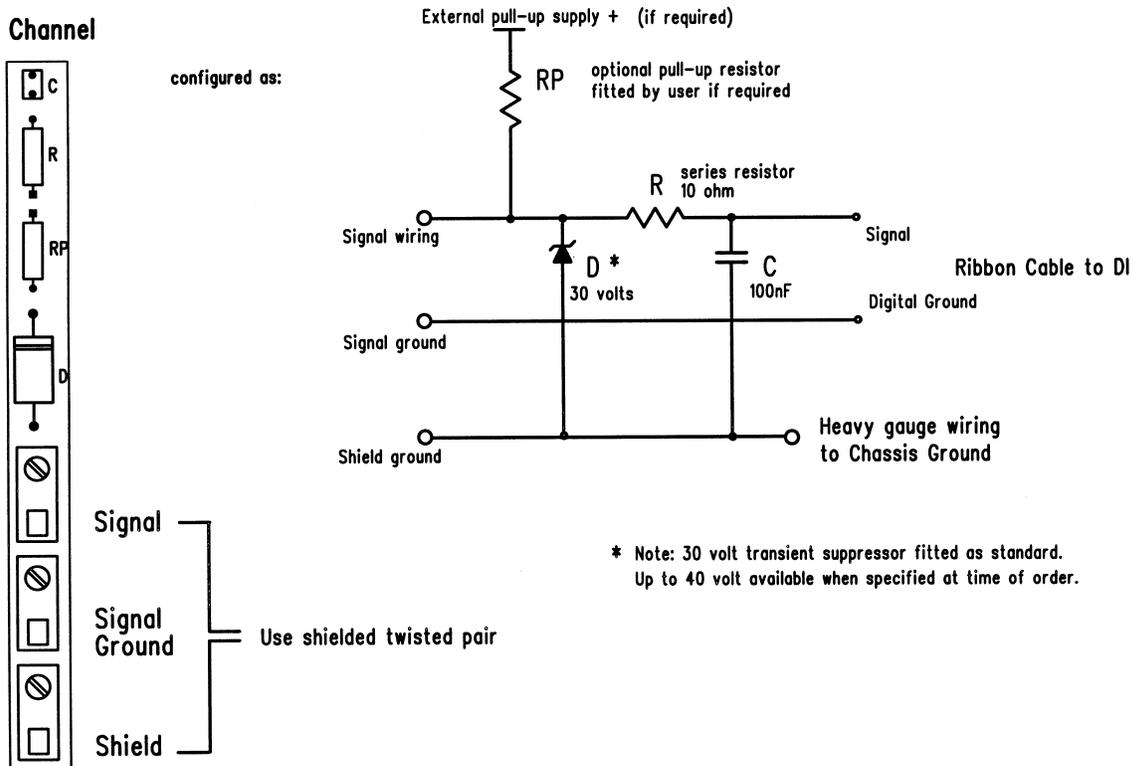
\* Note: 30 volt transient suppressor fitted as standard. Up to 40 volt available when specified at time of order.
