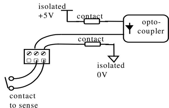
2) Loop powered. Some or all of the input opto-couplers can be set to be turned on by a signal loop applied externally. The two 330 ohm resistors must be removed from the positions labelled "contact", and one resistor of the correct value placed in the position labelled "LOOP". The current must flow into the terminal labelled "IN", and out of the terminal labelled "ret" (for "return"). The resistor value should be selected to limit the current flow through the opto-coupler to 10 mA or so.
