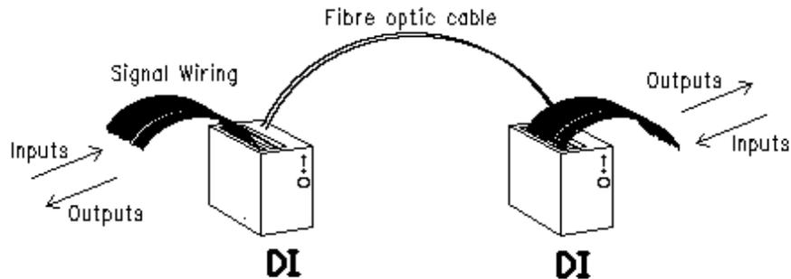
Group3 Device Interfaces connected with just two fiber optic cables provide noise free transmission of many analog and digital signals in difficult environments.
